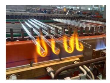
EVline is a family of systems designed to inspect glass tubes after the end-forming.
