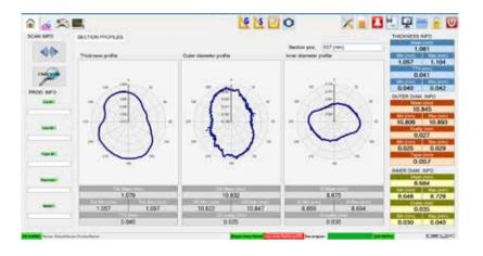
NIROX'S NCSIab automatic offline system is a powerful tool that quickly provides tubes measurements for quality control, quality assurance, inline machines qualification and supplier's incoming check.
