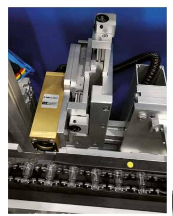
**Glass pharmaceutical primary packaging** must be produced under very **tight tolerance**. Dimensions must be 100% inspected to guarantee the **full-functionality of the packaging**. The bottom of the container plays a fundamental part for the integrity of the container during the filling process.
