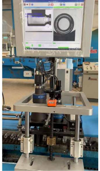
Visual inspection is nowadays mandatory equipment in a state-of-the-art tube converting production line. The VISIIne.D family of camera-based systems has been expanded to cover all inspection requirements directly on board in production line.
