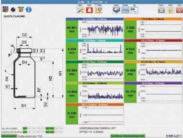
**Dimensional inspection** is usually performed **on the forming machine** when container is still mounted in a chuck. After this, there is the inspection before annealing oven, **on the afterforming line**, to **measure inner diameter and length**. Both are available **as a single station**.
